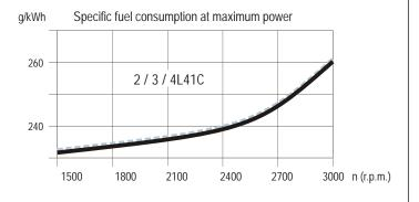
Performance data refer to Standard Reference Conditions of DIN ISO 3046: + 25 °C (77 °F), 100 m ALT, relative humidity 30 % During running-in period the output increases by approx. 5 % which is taken into conside- ration at delivery. Power reduction acc. to DIN ISO 3046. Standard values: Above 100 m ALT approx. 1 % per 100 m. Above 25 °C (77 °F) approx. 4 % per 10 °C (50 °F). The power taken from charging alternator also has to be added to the demand of power.
