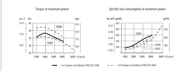
Performance data refer to Standard Reference Conditions of DIN ISO 3046: + 25 °C (77 °F), 100 m ALT, relative humidity 30 % During running-in period the output increases by approx. 5 % which is taken into conside- ration at delivery. Power reduction acc. to DIN ISO 3046.Standard values: Above 100 m ALT approx. 1 % per 100 m. Above 25 °C (77 °F) approx. 4 % per 10 °C (50 °F). The power taken from charging alternator also has to be added to the demand of power.
